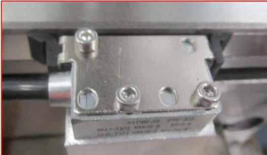
Tolerance of the gap between reader head and magnetic scale is 0.3mm to 1.0mm. This allows for any variance due to depth of groove scale is fitted in etc. Put a 0.5mm washer between the head and scale, tighten the 3 screws and remove washer.
